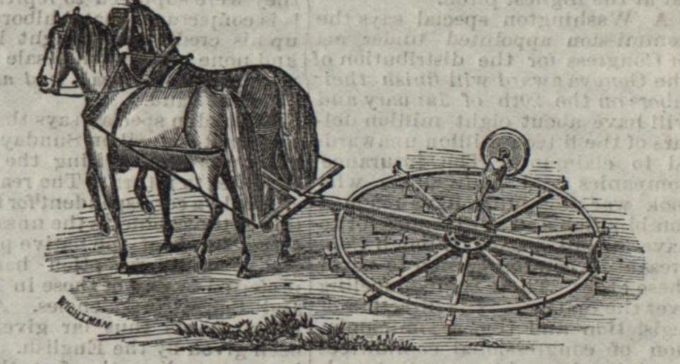
D EVOLVES continually while in operation so that large lumps or any obstruction of the kind cannot clog it. Therefore as a Pulverizer, Soil Mixer, Grain Coverer, and to Level the Surface it has no equal, doing three times the work of any other Harrow with same labor.
