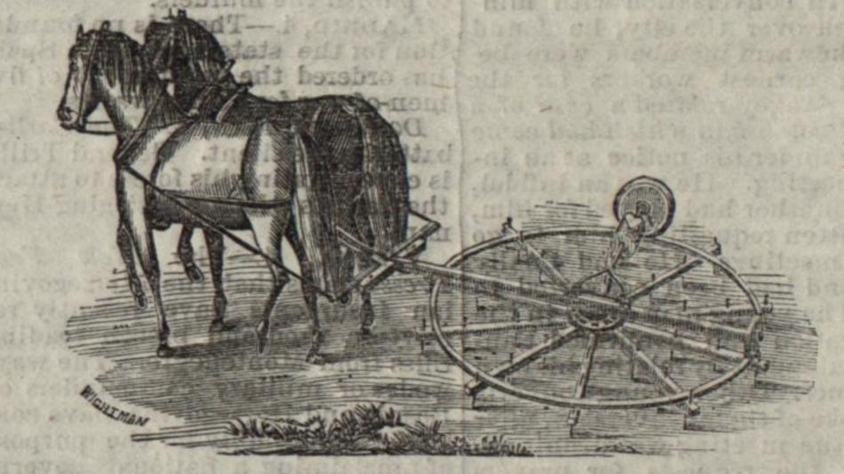
DEVOLVES continually while in operation so that large lumps or any obstruction of the kind connot clog it. Therefore as a Pulverizer, Soil Mixer, Grain Coverer, and to Level the Sur-
