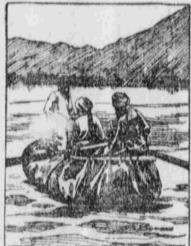
somewhat resembling that of a boat The contrivance was then attached to a cable stretched across the river, and passengers were thus ferried from one side to the other. The strange boat was waterproof and seemed to rest lightly on the surface of the river, Numerous smaller craft of the same construction were in common use by the natives. The yak is the most useful animal in Tibet. It is easily domesticated and is the burden bearer of the country.
