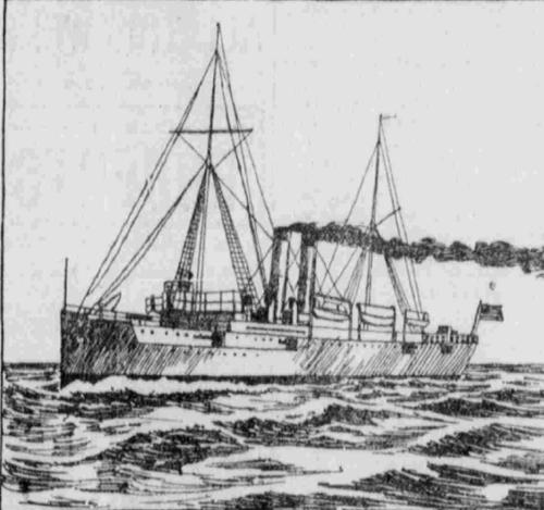
The Galveston was one of six vessels to be built under act of March 3, 1899 providing for protected cruisers of 2,600 tons trial displacement.
