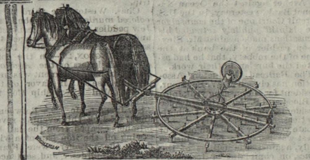
DEVOLVES continually while in operation, so that large lumps or any obstruction of the kind cannot clog it. Therefore as a Pulverizer, Soil Mixer, Grain Coverer, and to Level the Surface it has no equal, doing three times the work of any other Harrow with same labor. Thousands have been sold and are in use, giving the greatest satisfaction.
