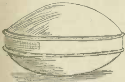
ONE OF THE COPPER BOILERS. (6 ft. 8 in. x 4 ft.)
