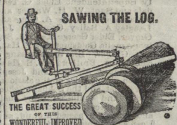
abor Saving RIDING SAW MACHINE is fully demonstrated by the number in use and the present demand for them. It saws Logs of any size. One man can saw more logs or cord wood in one day and easier than two men can the old way. It will saw a two foot log in three minutes. Every Farmer needs one. Township agents wanted. Send for
