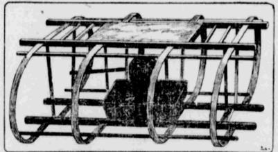
The curious device herewith illustrated was the forerunner ing pan. It consists of a wooden framework in the center of which is the brazier for charcoal. The framework was designed to keep the brazier from the bedelothing. There are several specimens of this quaint relic in American
