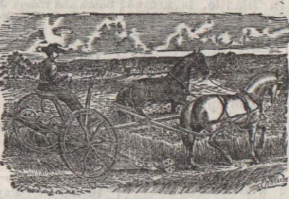
It will cut 6 feet easier than any SIDE-CUT Mower will cut 4 ) Average draft of 19 Side-cut mowers per foot, 44.63; Eureka only 28.66. I have examined the machine and talked with those
