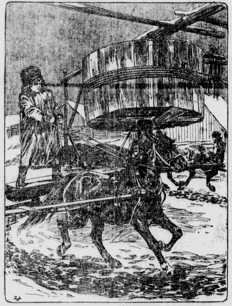
As may be seen from the cut, the horse winlass for drawing the ore from the mine is still used in the gold mining districts of the Ural.
